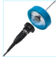
Step 2: Attach the camera. Connect camera onto the camera drape holder and extend the drape over the cable by pulling back the ring. Any excess drape is retained inside the ring.
